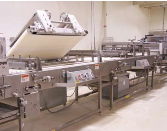
▲ The bakery's new bread forming line employs the latest advances in sheeting and pressure board technology.
