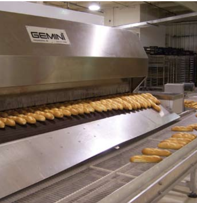
▲ A 60-ft tunnel oven now bakes the majority of Liscio's signature Italian bread and rolls, creating a crispy outer crust and tender inside crumb.
