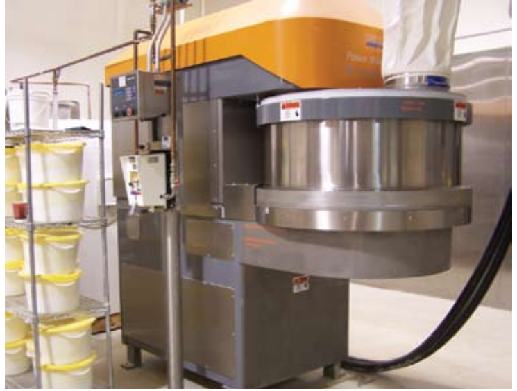
▲ "Telescoping" up and down to receive hand-adds, the spiral mixer's bowl also uses a release tool to drop finished dough into a mobile trough positioned below.
